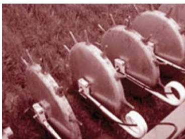
Spoke wheel injection places fertilizer in the root zone and is less susceptible to volatilization.
