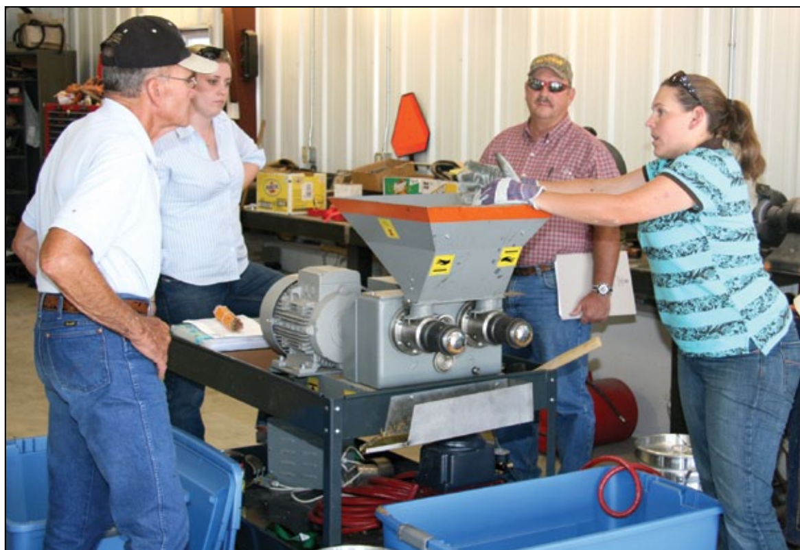
Extension educator Lindsay Taylor demonstrates a portable machine that presses oil from oilseed crops and can be processed into biodiesel.
