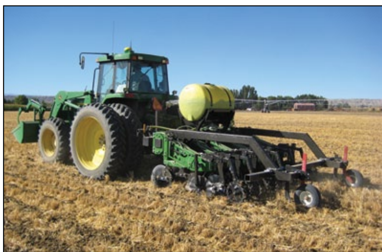
Fertilizer can easily be applied at two depths when the field is strip tilled.
