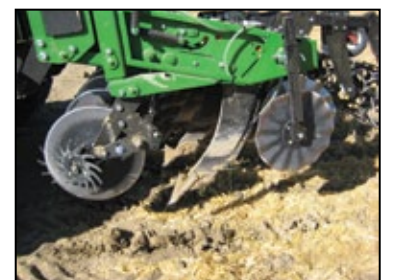
Front coulters cut the residue, and trash cleaners sweep residue away from the center. The shank rips a slot in the soil and places fertilizer. Fluted gathering coulters pull soil back over the slot, and the rear basket conditions the seed bed.
